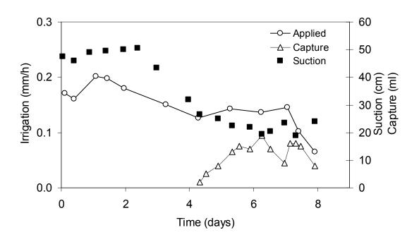
Fig. 3. The rate of drip irrigation applied to the drum, the capture rate of water in the WFD and the soil suction at the depth of measurement of the WFD.
