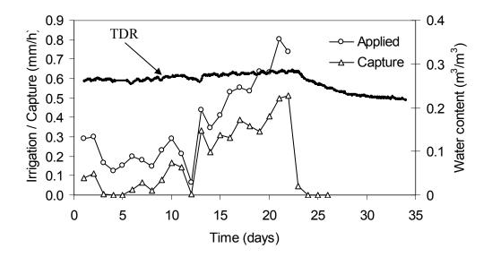
Fig. 2. The flux of sprinkler irrigation applied to the drum and the capture rate of water in the WFD. The heavy line shows the change in volumetric water content as measured by time domain reflectometry.
