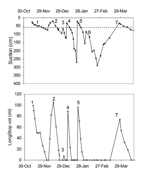
Fig. 4. The soil suction in the 'wick' of the LongStop (top) and the volume of water in the LongStop (bottom). The horizontal dotted line in the top graph demarks the theoretical sensitivity limit of the LongStop, above which the WFD should contain water. The numbers refer to the seven irrigation or rainfall events.
